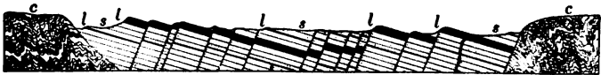
FIG. 315. Section of Triassic Sandstones of the Connecticut Valley ss , sandstones; l , lava sheets; cc , crystalline igneous and metamorphic rocks
